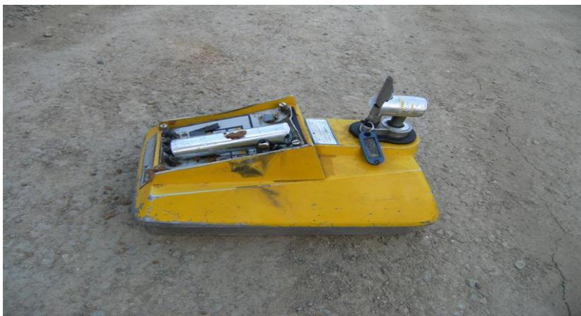
Transport box for a Troxler soil/moisture gauge with its content
