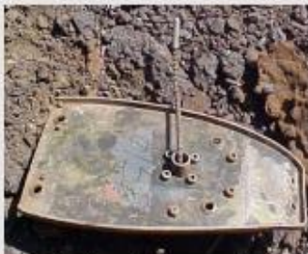
Damaged radiography camera with 'pigtail' (Iridium-192) 1 December 2003
