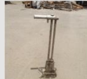
Damaged soil density gauge (Cs-137) 3 November 2010
