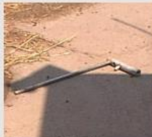
Damaged soil density gauge (Cs-137) 30 March 2004
