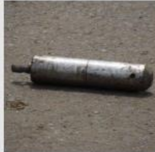
Damaged soil density gauge rod (Cs-137) 4 October 2010
