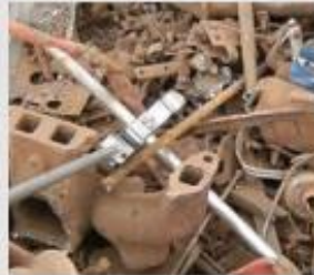
Damaged soil gauge rod (Cs-137) 14 May 2011
