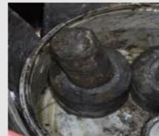
Lead source pin for density gauge (Cs-137) 20 July 2009
