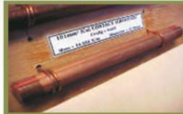
Contact Wire 161mm 2 : Unit made from copper
