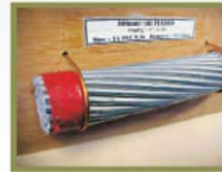
Feeder Wire 500mm 2 : Unit made from aluminium
