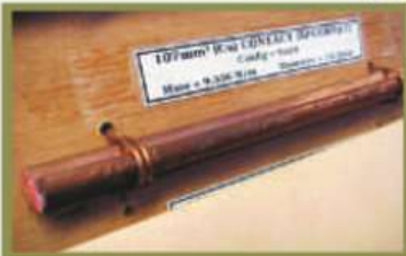
Contact Wire 107mm 2 : Unit made from copper
