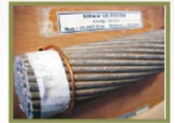
Feeder Wire 800mm 2 : Unit made from aluminium
