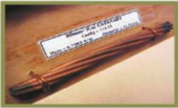
Catenary Wire 80mm 2 : Unit made from copper
